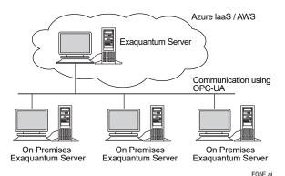
figure On premises Exaquantum and Exaquantum on cloud
