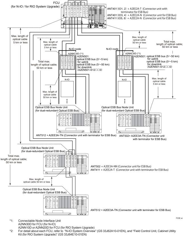
Figure Example of Chain and Star Connection (In the case of FCU for N-IO or FCU for RIO System Upgrade)
