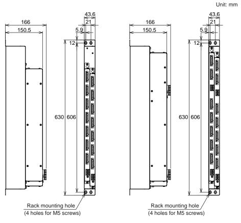
In the case of AEPV7D-10□, AEPV7D-20□
