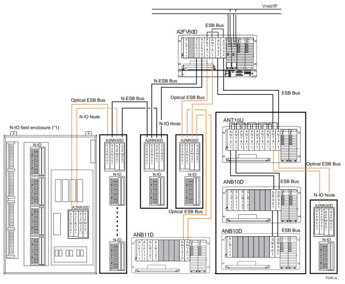
N-IO: I/O Unit for N-IO ANT4□1: ANT4□1-□E, -□F
