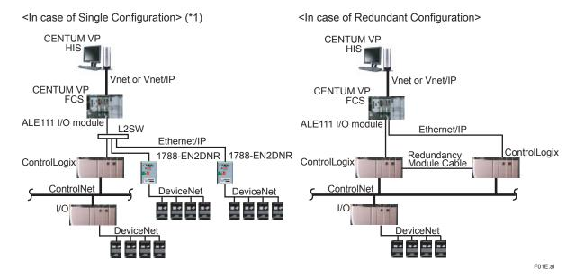
\*1: Single ControlLogix PLC and 1788-EN2DNR DeviceNet linking devices can be connected on the same EtherNet/IP network sharing the same ALE111 module as described above.
