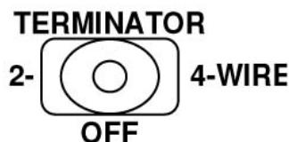
Figure 2.5 Terminating Resistor Selector Switch of the Module
