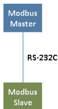
Figure: Modbus over serial line
